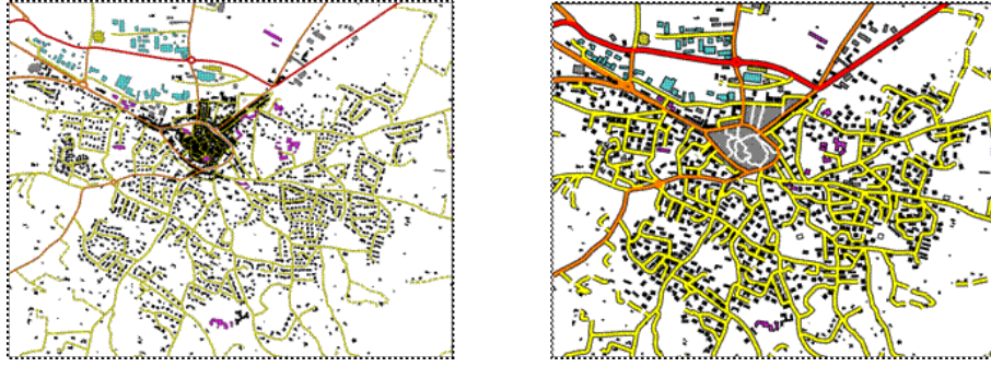
Figure 5: Generalization of topographic data from the IGN France BD Topo® database (reference scale 1:15 000) to a 1: 50 000 map. Result obtained with the AGENT model [Barrault et al., 2001].
